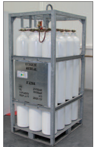
Oxygen high pressure cylinder rack 12 x B50
